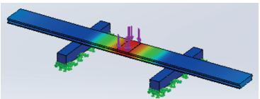
The calculations and tests of the breaking load values of the decks according to different tree types and thicknesses were carried out with the help of Novawood Test Systems in the Mechanical Laboratory of Manisa Celal Bayar University. Ergonomic and safe maximum stretching value of 1 mm (one) is accepted.
